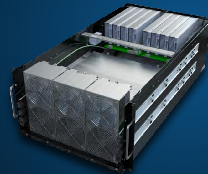
6U Gen 5 PCIe Expansion (up to 16 double-width GPUs)
